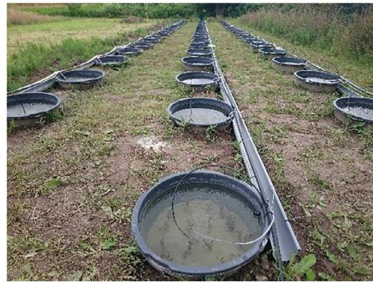
**Fig. 1.** Mesocosm design. Each mesocosm contained 24 L sediment (5 cm depth) and 50–55 L tap water (20–23 cm water level). An air pump was used for aeration of the mesocosms and fresh water was supplied via a tap water tube connected to a water hose. Excess water went through an overflow tube and into a gutter.
